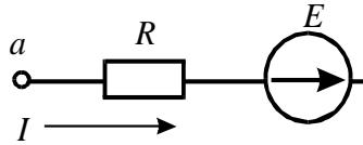
$I = \frac{\varphi_b - \varphi_a + E}{R} \quad 2)$ $I = \frac{\varphi_a - \varphi_b - E}{R} \quad 1)$ $I = \frac{\varphi_b - \varphi_a + E}{R} \quad 3)$ $I = (\varphi_b - \varphi_a + E)R \quad 4)$ |
